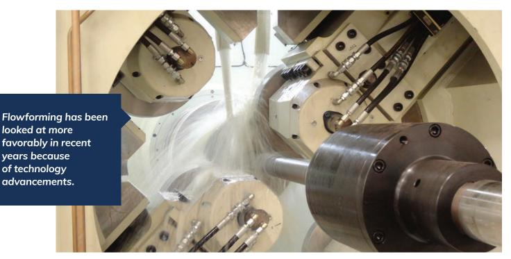
Also, flowforming has the ability to form many different types of materials. Typical applications include materials such as inconel, hastalloy, columbium and stainless steel (austenitic, ferretic and pH type).
