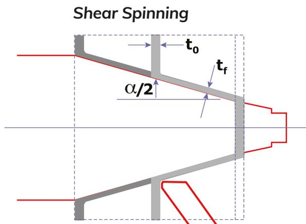
where  $t_f$  is the final component thickness,  $t_o$  the initial preform thickness, and  $\alpha/2$  the mandrel half-angle. When shear forming is done following the Sine Law, the primary deformation mode is pure shear, as opposed to tube spinning, in which more complex deformation modes occur.
